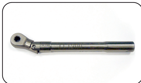
Wrench that has been disengaged upon reaching 200 Ncm
